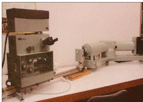
Figure 2. A laser microprobe. On the left – a laser microanalyser head, on the right – a Q-24 spectrograph for spectrum registration
