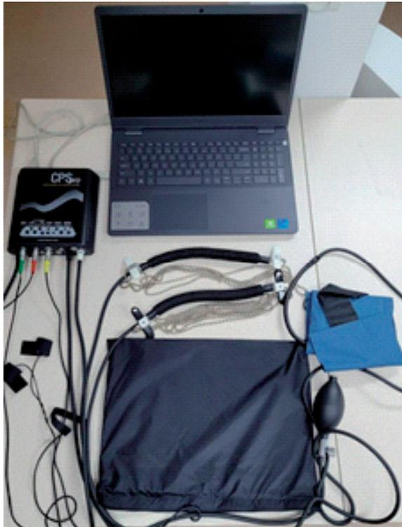
**Figure 1.** An example polygraph setup comprising a CPSpro – Stoeltinga and Dell mobile PC
